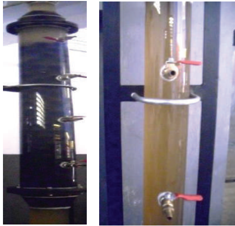
Figure 5. Process of Seeding-Acclimatization of Bioball Media HUASB Reactor
